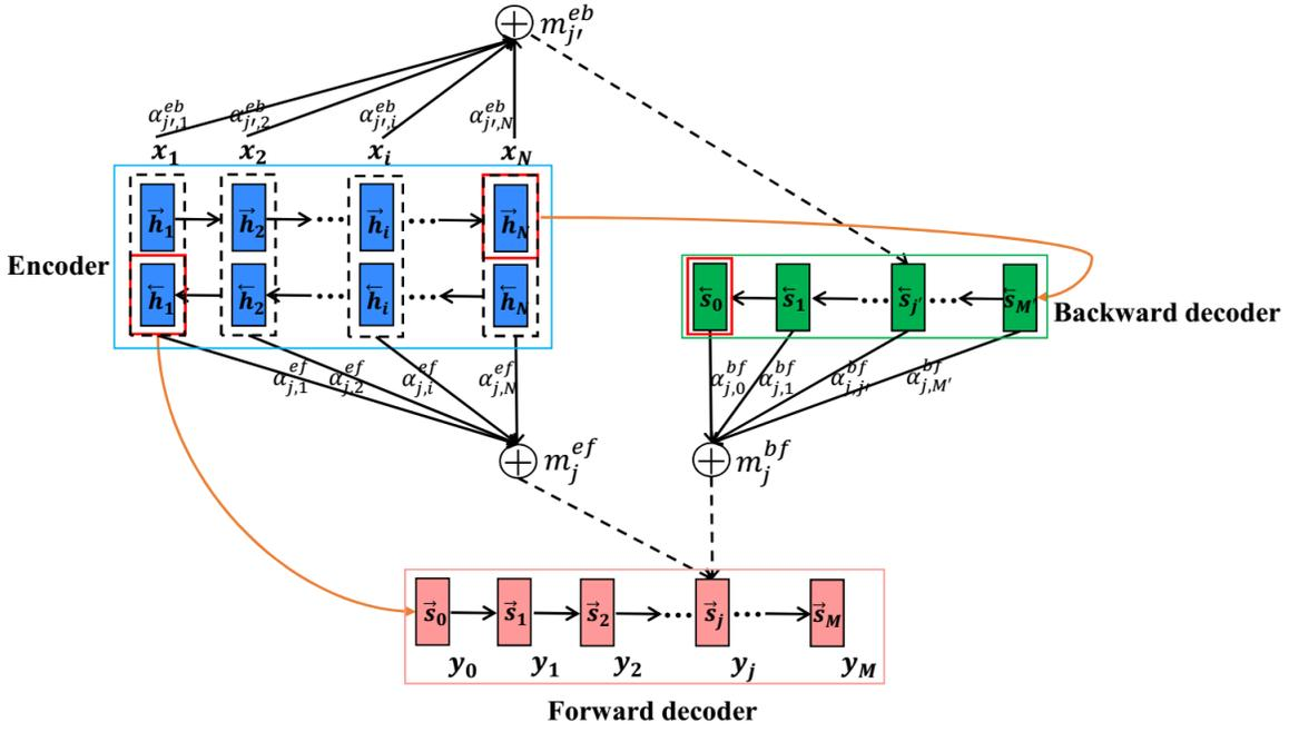
Figure 1: The architecture of the proposed NMT model. Note that the forward decoder directly attends to the reverse hidden state sequence  $\overleftarrow{s} = \{\overleftarrow{s}_0, \overleftarrow{s}_1, \dots, \overleftarrow{s}_{M'}\}$  rather than the word sequence produced by the backward decoder.
