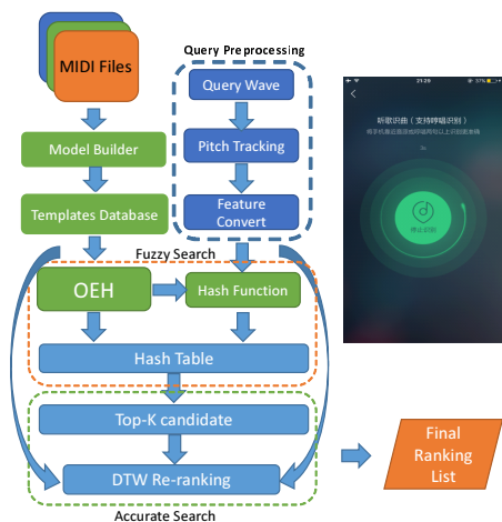
Figure 4: Framework of the Query by Humming.
